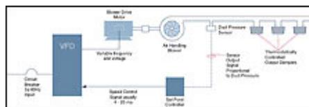
Figure 1: Simple Variable Air Volume Control
