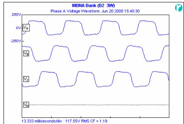
Figure 2: Voltage Flat-topping caused by 3<sup>rd</sup> Harmonic Blocking Filter
