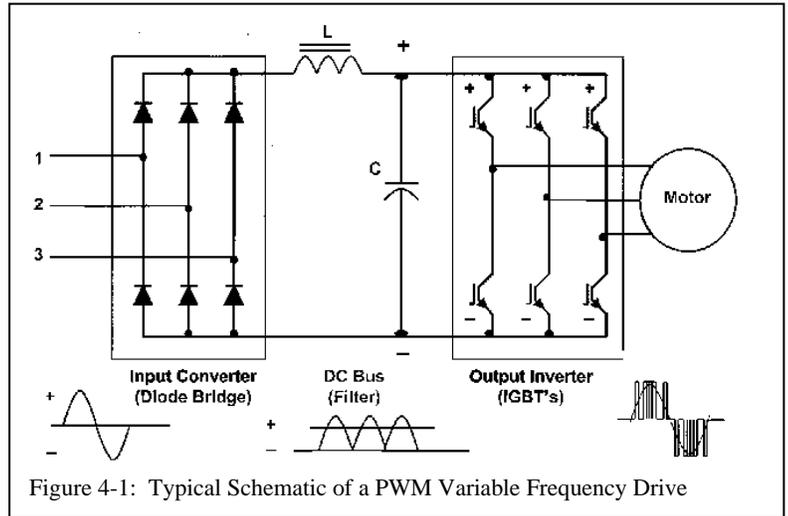
Figure 4-1: Typical Schematic of a PWM Variable Frequency Drive
