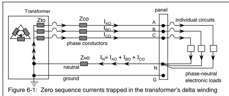
Figure 6-1: Zero sequence currents trapped in the transformer's delta winding
