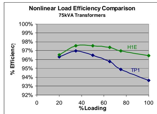
Figure 2: Non-linear load efficiency comparison
