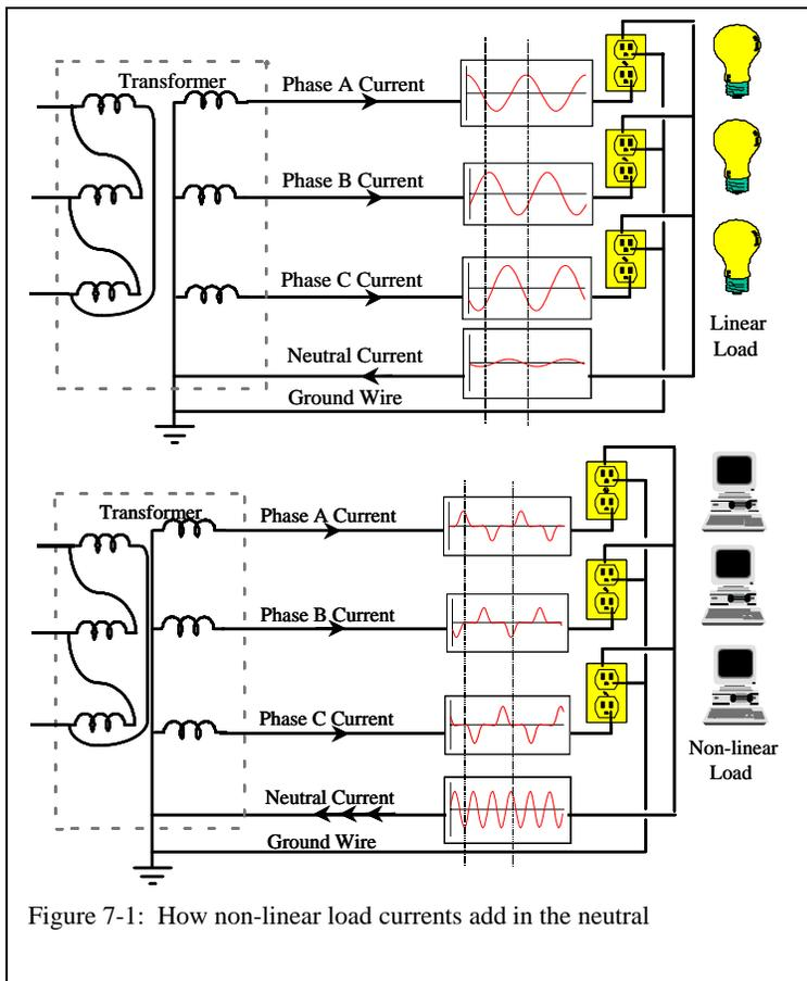
Figure 7-1: How non-linear load currents add in the neutral
