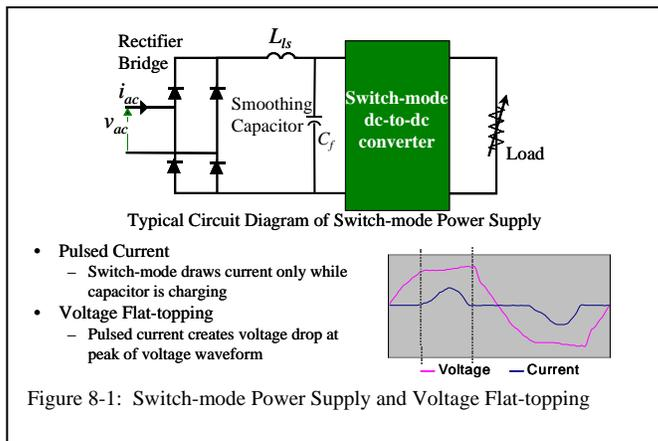
Figure 8-1: Switch-mode Power Supply and Voltage Flat-topping
