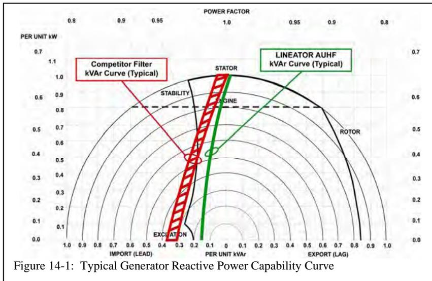
Figure 14-1: Typical Generator Reactive Power Capability Curve
