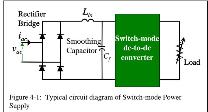
Figure 4-1: Typical circuit diagram of Switch-mode Power Supply
