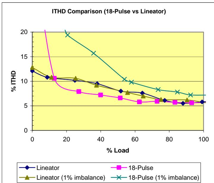
Figure 12-1: Input Current Distortion comparison – 18-Pulse vs
