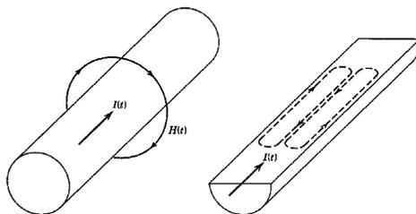
Figure 3: Skin effect in a conductor<sup>3</sup>
