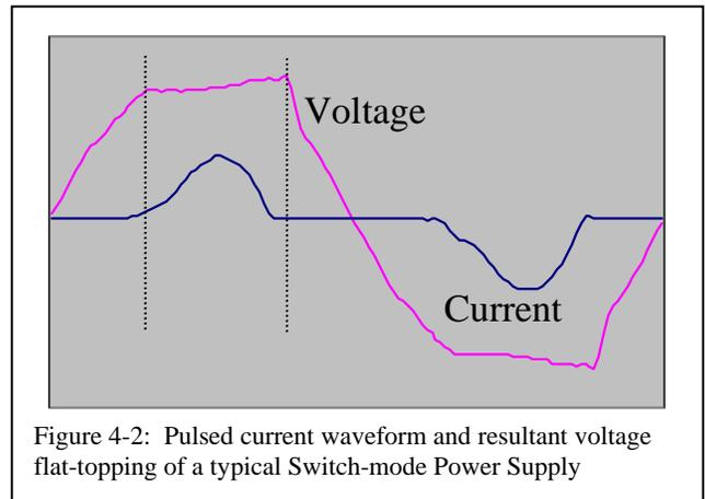
Figure 4-2: Pulsed current waveform and resultant voltage flat-topping of a typical Switch-mode Power Supply
