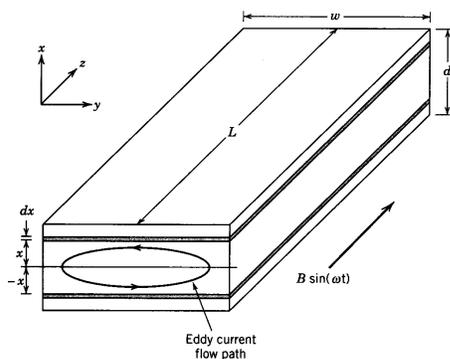
Figure 4: Eddy currents in the steel laminations of a transformer<sup>3</sup>
