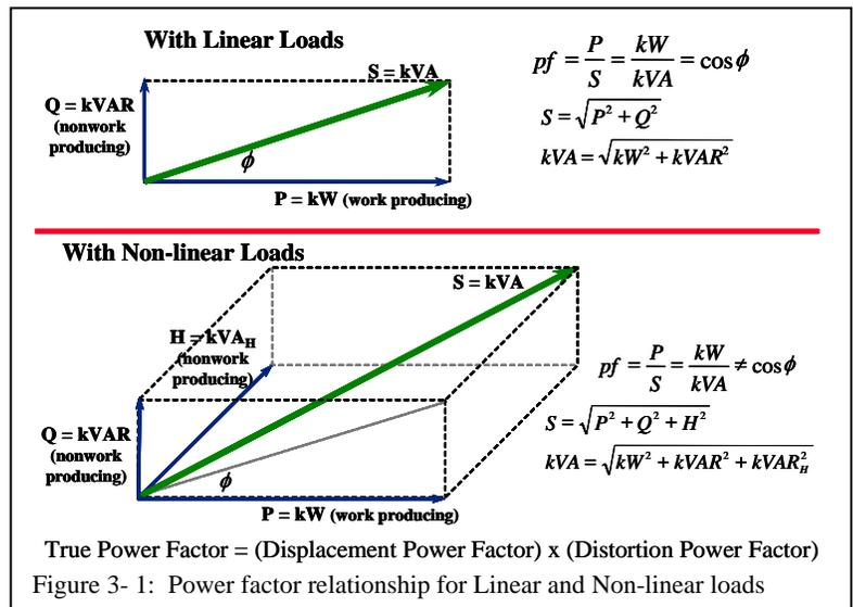
Figure 3- 1: Power factor relationship for Linear and Non-linear loads
