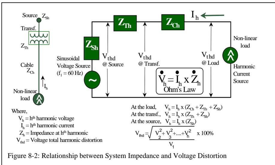
Figure 8-2: Relationship between System Impedance and Voltage Distortion
