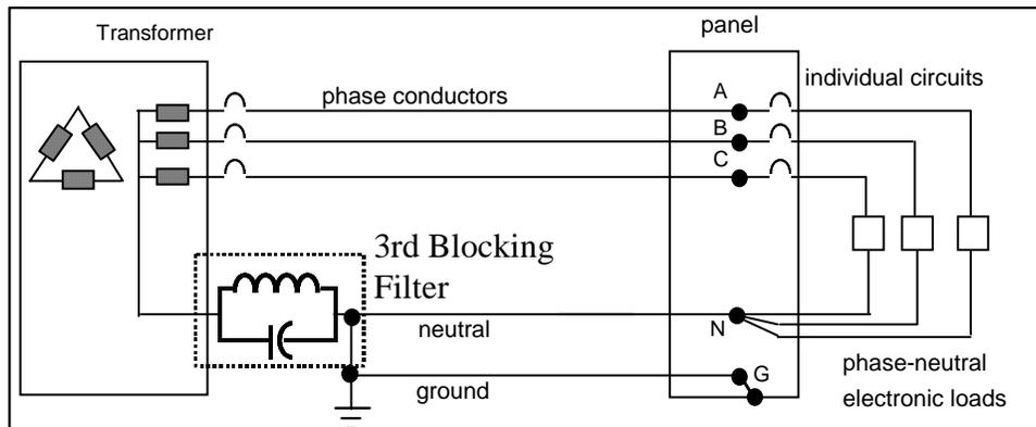
Figure 14: Typical installation of 3<sup>rd</sup> Harmonic Blocking Filter
