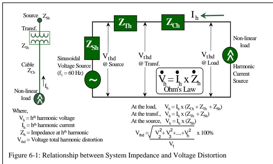
Figure 6-1 shows the relationship between system impedance and the voltage and current distortion components at several points in a typical power system.
