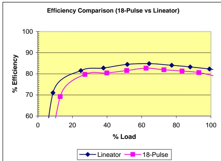
Figure 12-2: Efficiency comparison – 18-Pulse vs LINEATOR™/6-Pulse combination
