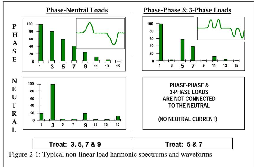
Figure 2-1: Typical non-linear load harmonic spectrums and waveforms
