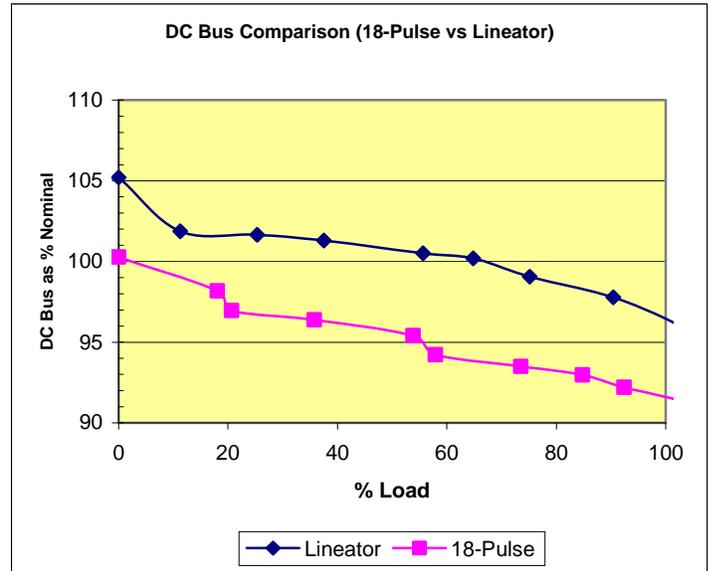
Figure 12-3: DC Bus Voltage comparison – 18-Pulse vs
