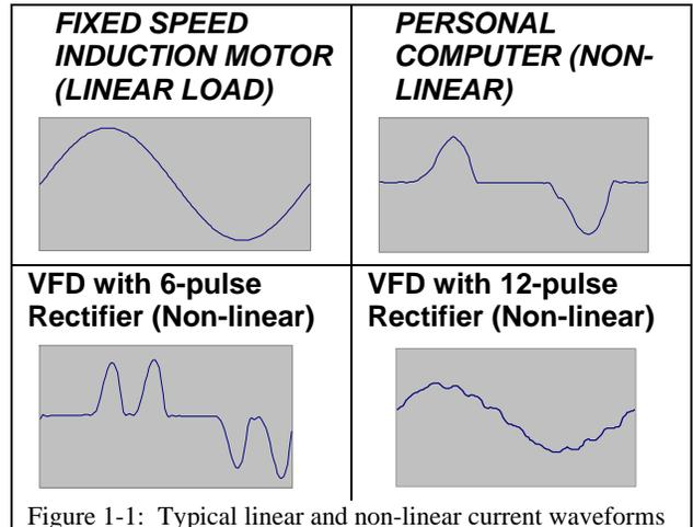
Figure 1-1: Typical linear and non-linear current waveforms
