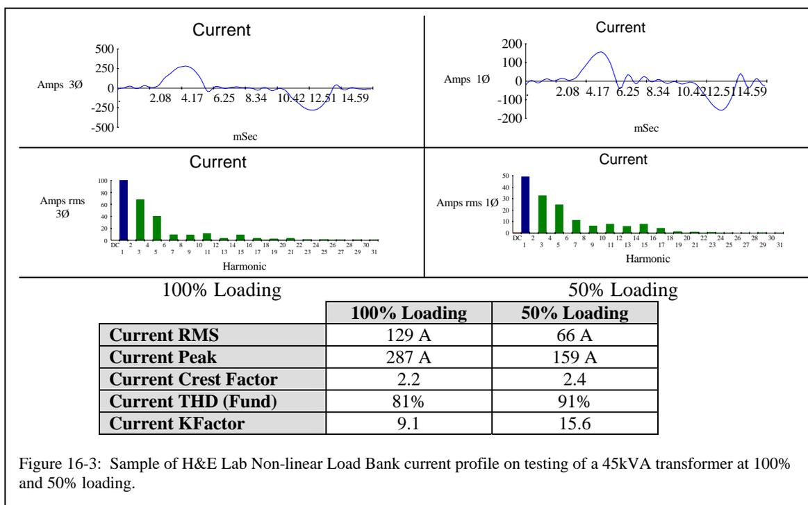
Figure 16-3: Sample of H&E Lab Non-linear Load Bank current profile on testing of a 45kVA transformer at 100% and 50% loading.
